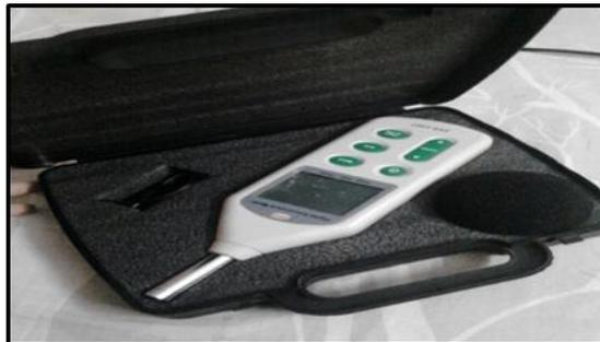
Figure 1.1 Digital Sound Level Meters
